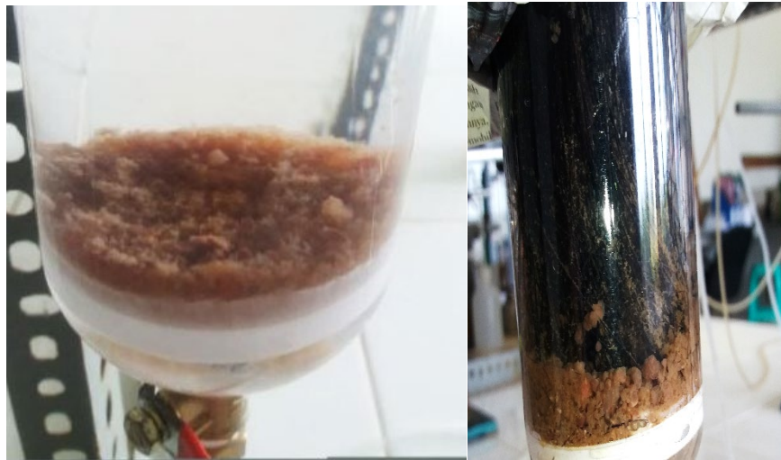
Figure 2. Anammox granular as seeding sludge (a) and palm fiber as the carrier (b) for start-up reactor.
