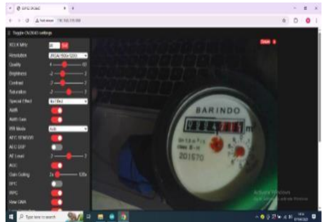
Figure 2. ESP32-CAM live stream output and parameter control interface.
